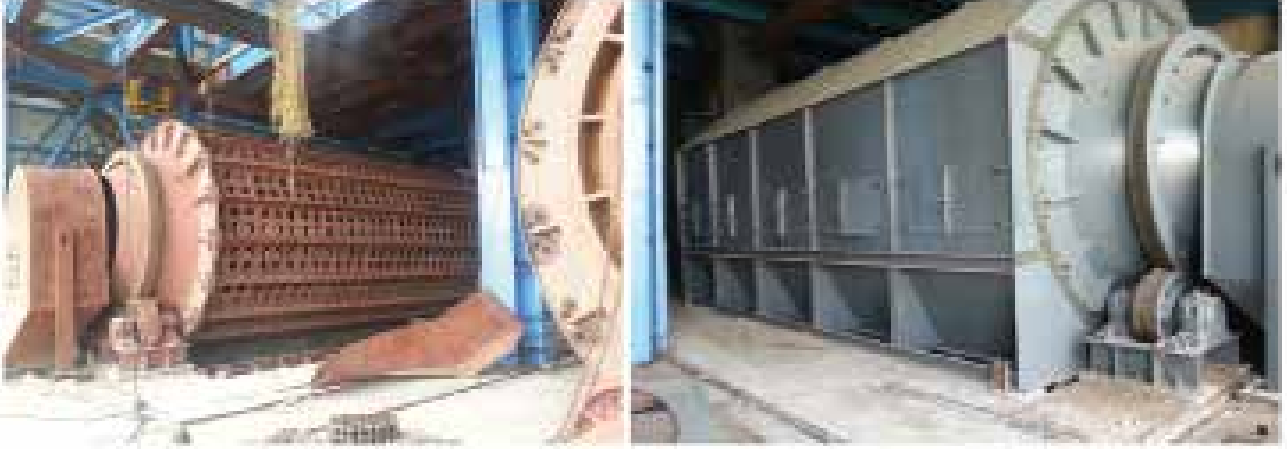
Rotary Breaker for Coal Handling Plant, Mettur, Tamil Nadu - India
